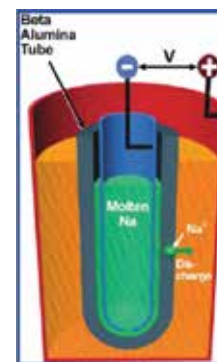
Figure 18: Schematic representation of sodium-sulphur batteries
